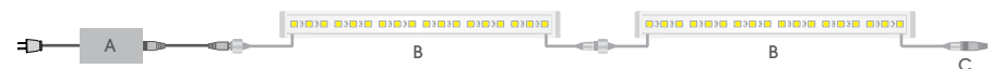
A. Power Supply: DL-PS-xx/24 B. LED Luminaire: DL-RS-xx-xx C. End Cap: DL-PS-OD-EC (required for outdoor use)
